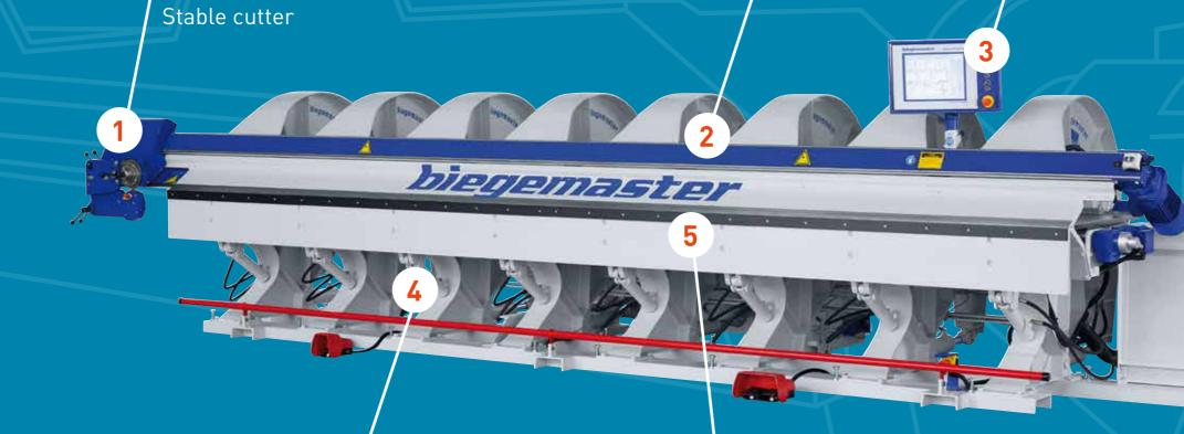
Hydraulically driven bending joints
