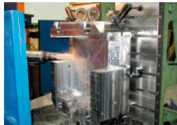
MILLING OF A TOOL FOR A FORM STAMPING
