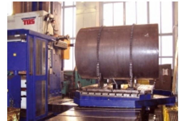
MILLING OF A FRONT ROLL FOR A ROADROLLER
