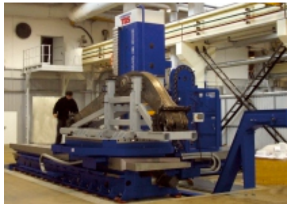
DOUBLE-SIDED MILLING OF A CRANE ARM
